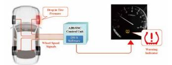
**Deflation Warning System (DWS)** \*DWS is a kind of tire pressure ( These systems analyze wheel speed signals from the rotation of tires to detect and notify the driver of decreases in tire air.
